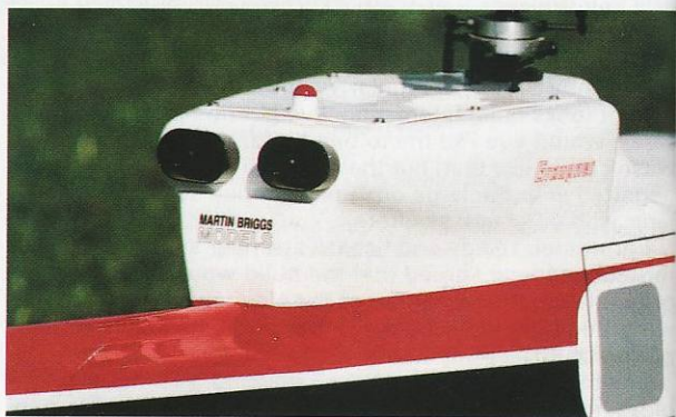
The large hatch behind the main shaft allowed access to the receiver, NiCad and four servos, controlling five functions through a rack of bellcranks. This model also has a gyro and an additional separate throttle servo, which probably has more power than the combined might that the original four may have had.
