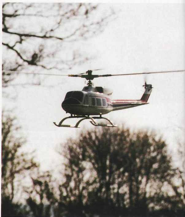
The tail rotor drive wire runs at engine speed with a 2:1 reduction in the gear-box. An external pitch slider, driven by a rod going through the tail shaft, gave fairly precise tail control to the wooden tail blades. Not as sophisticated as current designs, but the shorter tail shaft was less vulnerable in a crash.
