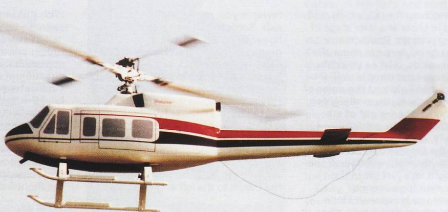
The crisp paint job really stands out well in bright sunshine. Just look at that coning-angle, a combination of built-in sweep and a very slow rotor speed (between 11 and 1200rpm). I must do something about that sagging piece of aerial wire!
