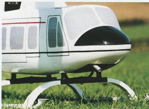
Unscale but wide-base undercarriage gave a little more ground stability but most beginners fitted the optional inflatable float set to give even wider stance and to absorb those inevitable landing shocks. The undercarriage cross-struts were made from multi-laminate wood and were bolted to the fuselage via rubber shock-mounts. The silencer (!) outlet position is unusual but does in fact keep the model quite clean and free of the exhaust residue that used to contain the gooey remains of castor oil - which was about all we had as lubricant in those days.
