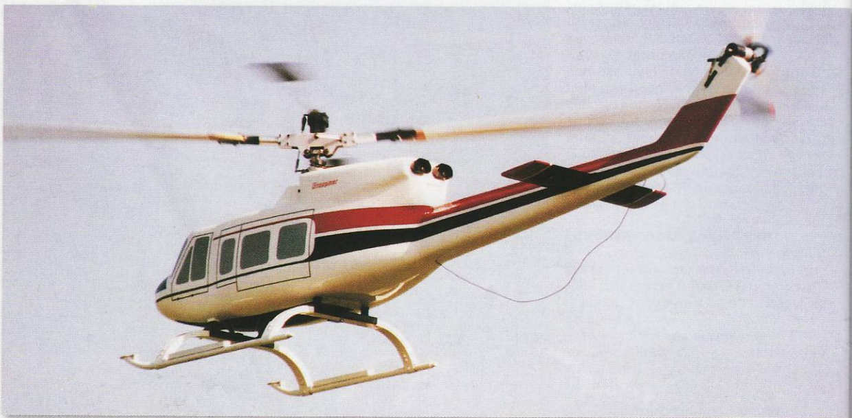
The large hatch behind the main shaft allowed access to the receiver, NiCad and four servos, controlling five functions through a rack of bellcranks. This model also has a gyro and an additional separate throttle servo, which probably has more power than the combined might that the original four may have had.
