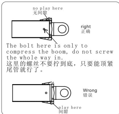
Make sure the Boom is pushed to the bottom of the Gear Box before tightening up the M2.5 Bolt. 先将尾管插到齿轮箱底部再用M2.5螺丝上紧。
