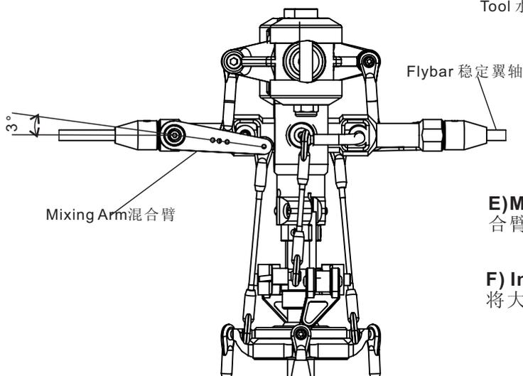
**E) Mixing Arm is set 3deg down to the flybar. 混合臂设为3度于稳定翼轴**
