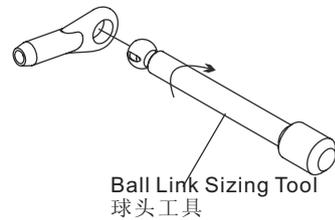
Be aware that the Ball Link Sizing Tool is very sharp. Do not oversize the ball link.
