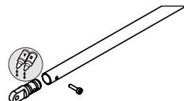
Apply AB Glue on Boom Support. 尾撑杆接头处用环氧胶粘好.
