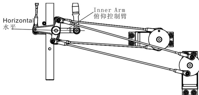
**c) Next adjust the links from T Arms to Swash Plate to level Swash Plate. A compass Swash Plate Tool can be applied here as a guide.**
