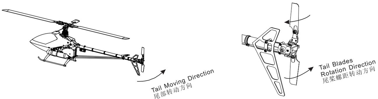
5. Check that the Main Blades, Paddles and Tail Blades are installed in the right direction. 检查大桨,平衡翼及尾桨的安装方向是否正确.
