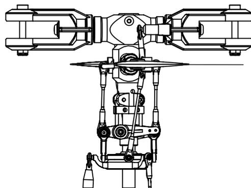
Leave About 0.1mm Play between the flybar collar and the flybar holder. This could reduce the chance to snap the flybar when flying.
