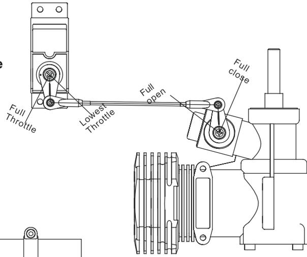
**H) At Rudder Middle Stick, Set Rudder Servo 90 degree to the tail link And Set Tail Blade to 7 deg Pitch.**
