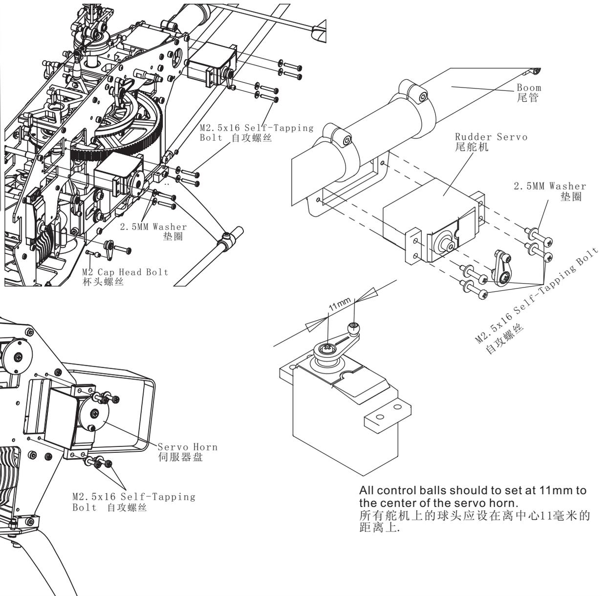
All control balls should to set at 11mm to the center of the servo horn.
