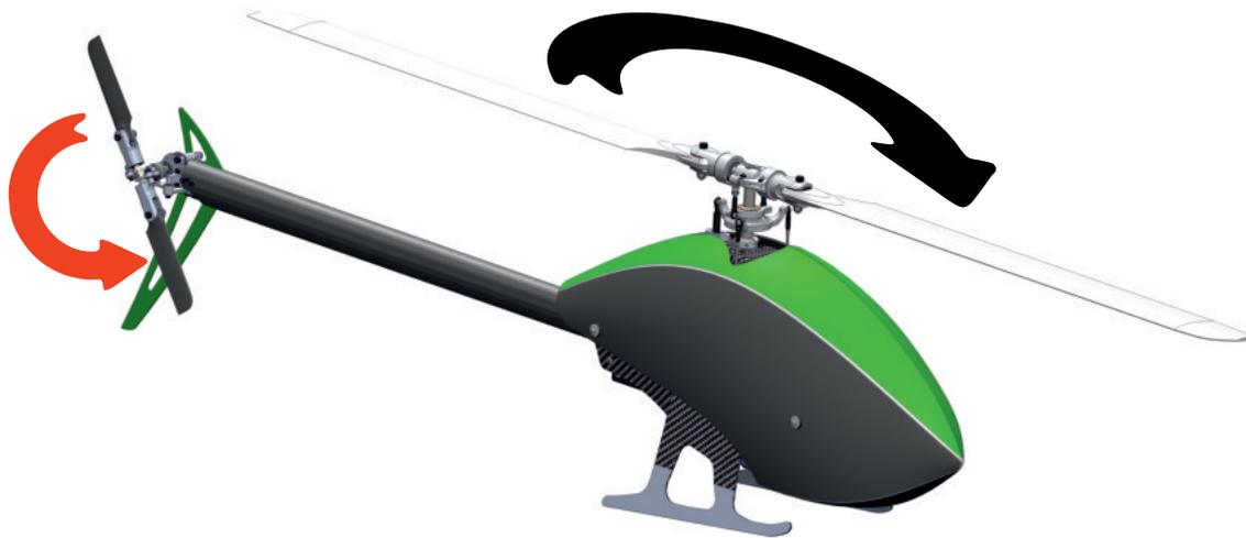
**When main rotor rotates clockwise (black arrow) tail blades should rotate counter clockwise (red arrow)** as observed from right side of the helicopter. If not, the belt is twisted in the incorrect direction (see step 15). Be sure that main rotor and tail rotor blades are installed in the correct direction.
