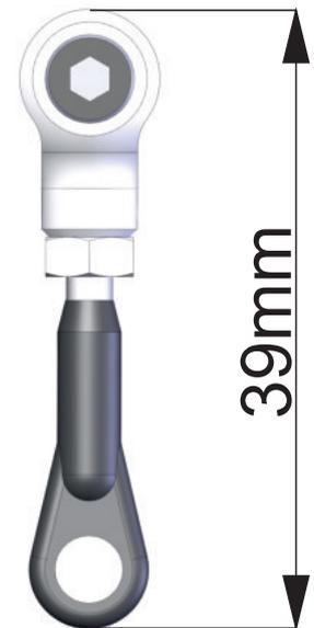
Press bearings (5) into Swash driver (1). Don't forget to put drive collar (2) between the bearings. Mount set screw (8), hex nut (9) and ball link (6) to swash driver (1). Slide bolt (7) through washer (3), swash driver and washer (4) and mount it to parts from STEP1 (10). Length of whole swash driver assemblies (outside to outside) should be 39mm.
