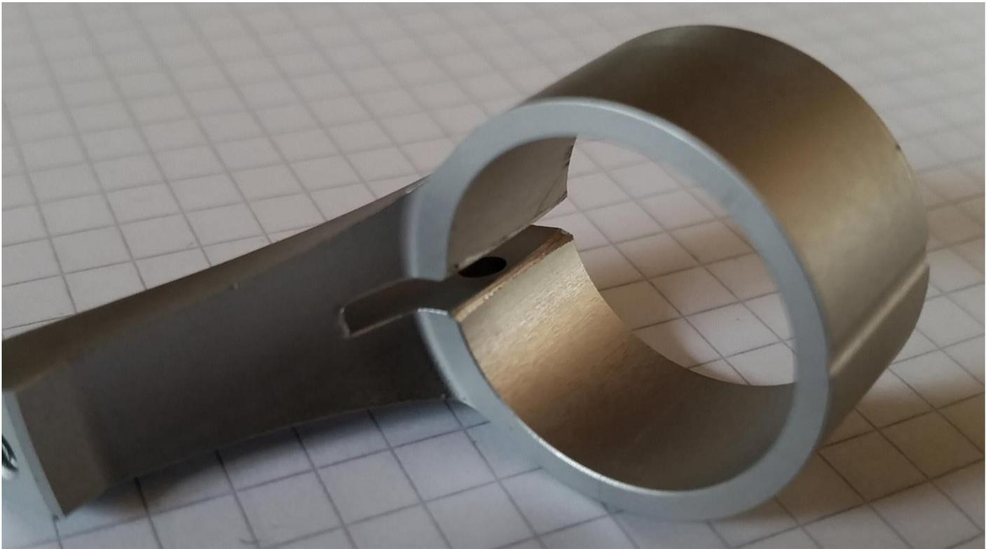
Please be careful while assemble the arm to the blade grip. There is a marker on the arm and the grip to show you the center position. It should not look like this but perfect centered! Also do not over tighten the bolt. There is not much pressure necessary to clamp the arm save!
