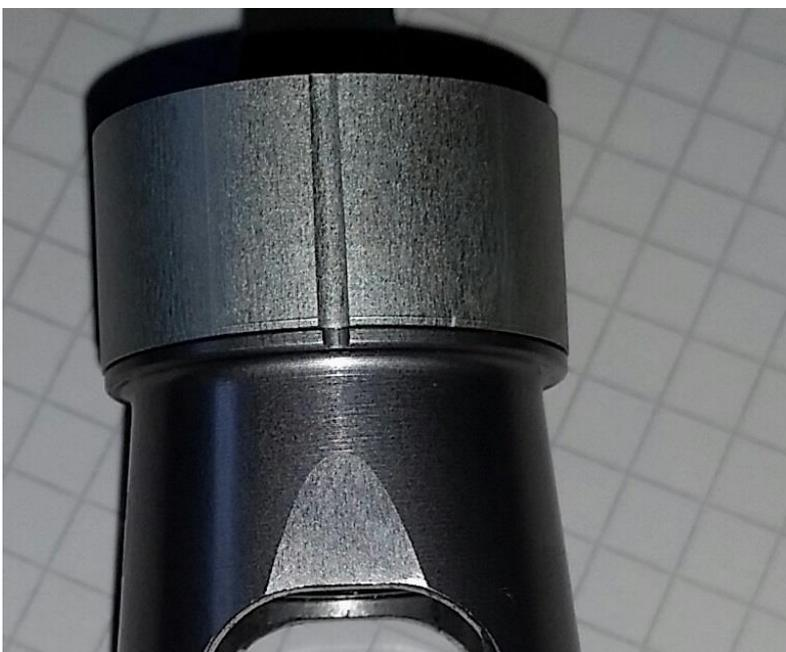
This pictures showing the new blade grip arms and blade grips coming soon! You can see that we add a lot of material. It is also increasing the rotor diameter by in total 4mm. We moved the hole position because of the coming three blade rotor head (to fold in the blades easier). Green is the new one.
