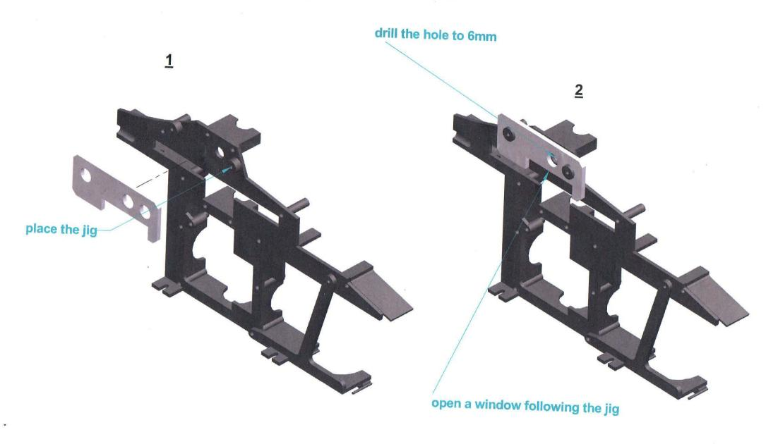
MAKE THESE OPERATIONS ON BOTH PARTS OF THE MAIN FRAME
