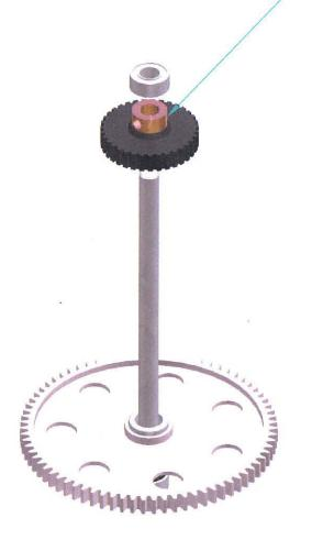
leave a little distance (0,2-0,5 mm) between the bottom of the pulley and the main gear
