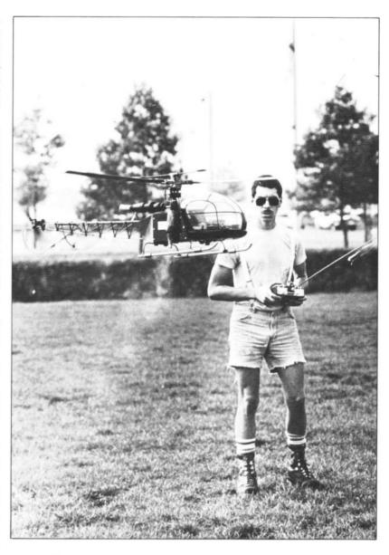
streamlined shape, seems to move more cleanly in forward flight than an Allouette, which has a large canopy. Tail rotor response is also more smooth than with a standard Allouette.
