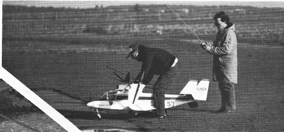
Left: 1/7 scale Bell XV15 Tilt wing VTOL aircraft by France's Georges Chaulet. Model is 8ft. wide over rotors and weighs 10lb for OS90 power. Rotor angle is fixed and the model is flown as an autogyro. Above: Georges prepares the model for take-off while a friend holds the transmitter.
