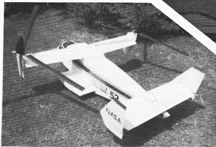
Left: 1/7 scale Bell XV15 Tilt wing VTOL aircraft by France's Georges Chaulet. Model is 8ft. wide over rotors and weighs 10lb for OS90 power. Rotor angle is fixed and the model is flown as an autogyro. Above: Georges prepares the model for take-off while a friend holds the transmitter.
