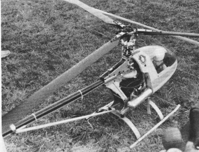
Left: John Barrows 3 bladed rotor head on the Kalt Baron (see text for details).
