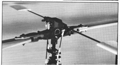
situation. Control movement increases don't always produce the required effect, the aforementioned paddle lightening exercise should be tried. Whatever modification is tried, full and careful hover tests should be conducted before trying the aerobatic manoeuvre. It may well be found that stiffening up the head can have unwanted side effects such as 'nodding' if the rotor rpm is too slow.
