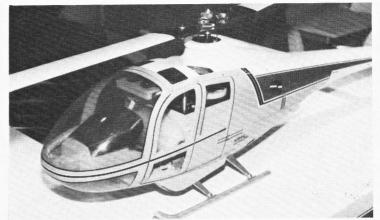
Lockheed 286L from Kavan, above, features a flybar-less rigid rotor type head.
