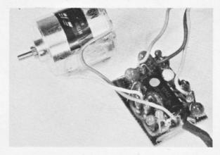
Slim shaped Sportsman receiver employs German Hirschman servo and battery connectors which very effectively support the leads at soldered
