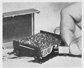
vibrator with a preset potentiometer in each of the timing circuits. In fact, we still have a total of 13 preset pots in the Tx. as before, very good for quick setting up but perhaps not very 'finger-proof'.
