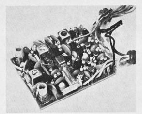
Above left: the receiver crystal is also removable for quick change of operating frequency. Small receiver crystal unit is easily handled, thanks to plastic tag. Note how p.c. board is retained in case by lips which slot into case ends. Above, receiver component layout. Note position of crystal in socket.
