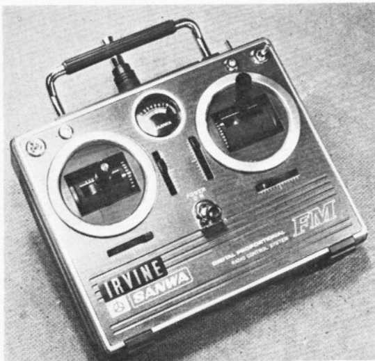
The cleanly 'different' lines of the transmitter are shown up well in these photos, while above close-up shows the adjustable-length sticks. Below: back removed to show p.c. and battery housing.
