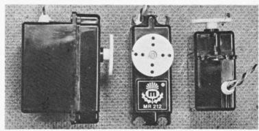
Out of its case, the printed circuit board, inverted to show neat design and workmanship. Note crystal-holder. At right: servo opened up to display gear train and electronics- plus16mm motor.
