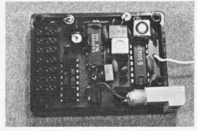
With and without lid-the receiver has three i.c.'s and two filters; bank of seven sockets has sprung contacts.
