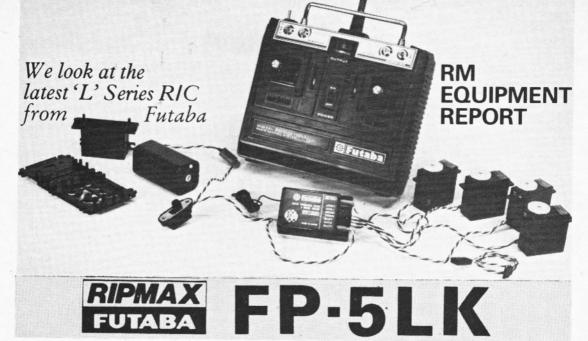
THE FUTABA "L" SERIES, based on the well proven "M" Series, features voltage stabilised circuitry for maximum efficiency when using drycells. The "Combo's" of the "L" Series are sold complete with drycell power pack containers (battery boxes) for initial economy but the systems are quite easily converted for use with rechargeable NiCads. A NiCad conversion set is in fact obtainable from RipMax stockists — a suitable charging unit is also offered.
