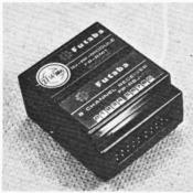
outputs and power and encoder input plugs. The whole is compact in design and strongly cased-those plugs and sockets being particularly small, neatly polarised and crimped onto the leads. Much attention is paid to screening, and the RF modules have ceramic filters and
