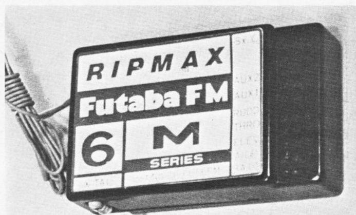
Above: FM receiver is similar in size and layout to the AM but crystal is differently positioned. The socket labelled SxC is for remote operation of a throttle servo via an accessory not yet available. Below: hefty helical output gears mounted on a robust shaft are features of the 26m servo.
