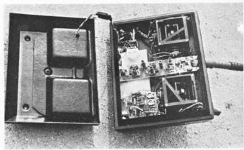
Above left: the short aerial is a simple plug-in item — users should make certain that the plug and socket are not allowed to become dirty. Above right: transmitter back removed to reveal the split 500 mAH battery pack in the case back, connected to the circuit board via a plug and socket. Central board is the RF section whilst smaller board in lower left hand corner (as seen in picture) is the encoder section.
