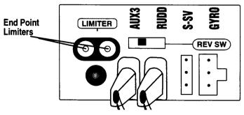
With your radio system on, give a full right rudder command. Using a small straight screwdriver, adjust the right potentiometer while noticing the rudder servo. Adjust the pot until the servo has maximum available travel but no binding occurs. Then give a full left rudder command and adjust the other pot to the point just before the servo binds. This sets the maximum available travel and eliminates linkage binding/over-stroking while the helicopter is on the ground.
