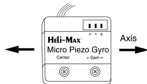
❑ 1. You can mount the gyro anywhere on your helicopter as long as its **rotation axis** (noted on the label on your gyro) is lined up with whatever
