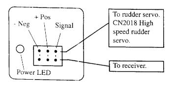
Warning, if any radio system is used other than JR or Futaba make sure same polarity is mantained otherwise you will damage the FG-01T.
