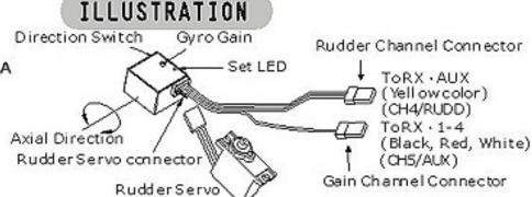
1. Use the adhesive foam provided to attach the gyro to the chassis of the helicopter. The foam will provide a stable, vibration free mount to securely attach the gyro to the helicopter. Align recommends the gyro to be mounted as illustrated in the diagram. If not possible, install it in a similar fashion, away from anyheat source or electrical source such as the motor, or ESC to avoid interference.
