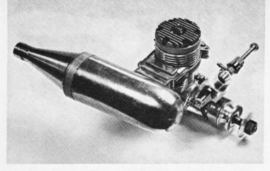
main transfer ports flanking exhaust, angled to direct gas to left side of cylinder and timed to open and close at 60 deg. each side of BDC. Rectangular third port, diametrically opposite exhaust port, chamfered to sweep gas upward and timed to open and close at 56 deg. each side of BDC.
