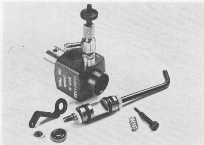
Tarno carburettor with throttle valve removed showing O-ring seals and 'clutch' parts. Extended manual control arm on opposite side enables throttle to be operated without switching on radio.
