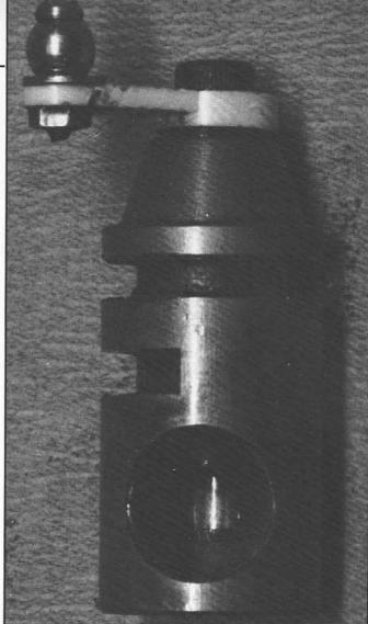
This view of the barrel clearly shows the metering device in the centre of the throat.
