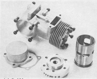
the other hand, is bigger but is open for a 4 degree shorter period. The Webra has a thicker walled cylinder liner than the O.S. (1.75mm instead of 1.2mm).
