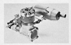
recovery. On larger props, steady idling down to less than 2,000 was obtained. Response to needle-valve adjustment was good. Using pressurised fuel feed increases needle response and a lower setting is necessary, of course, but the control remains non-critical.
