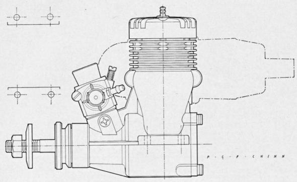
secured to main casting with six Allen type hardened chromium-molybdenum steel cap screws.
