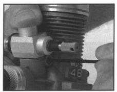
1.3 Once the carburettor is seated and aligned correctly, keeping pressure on the carb to hold it in place, tighten the pinch-bolt securely. Do not over tighten.
