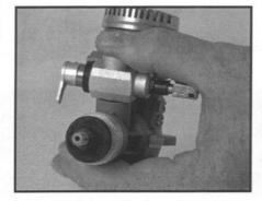
1.2 Next push down firmly on the carb to seat the carburettor and compress the Oring. A gap will allow excess air to leak in and affect the operation of your engine.
