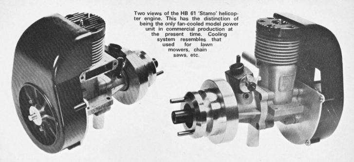
distributed in the U.K. by RipMax, the 'Stamo' fan-cooled version of the HB 61 is now available as a separate item for helicopters or, with a different flywheel, as an alternative to the water-cooled HB 61 for marine use.
