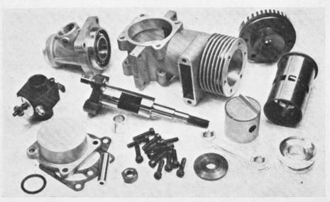
Parts of the HB 61. Differences between this and original Veco-Europe series include deletion of skirt transfer ports in piston and liner, a hardened instead of chromed, cylinder bore and a revised crankshaft. (All these mods. are also now incorporated in the Veco-Europe version.)
