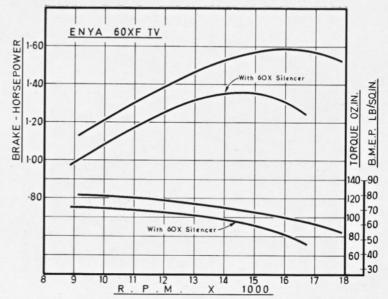
on the same fuel. In terms of prop speeds, losses due to the addition of the silencer ranged from only 400 rpm on the  $14 \times 6$  to some 700 rpm on the  $11 \times 7\frac{1}{8}$ .
