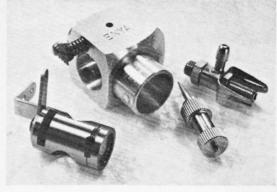
diametrically opposite exhaust port, angled to direct gas upward and timed to open and close at 57 deg. each side of BDC.
