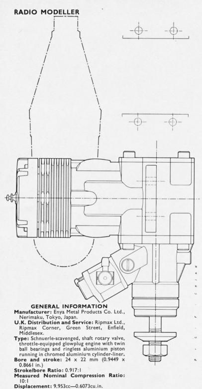
end of throttle barrel. Fuel conveyed to jet tube in throttle barrel via bypass channel in carb body and tapered grooves in surface of throttle barrel which meter more fuel as throttle is opened. Fine control of idle mixture by means of manually adjustable airbleed.
