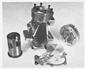
valve port timed to remain open from 40 deg. ABDC to 52 deg. ATDC. Shaft supported in one 15 x 28 mm. 10-ball steel-caged ball journal bearing at rear and one x 1/2 x 1
