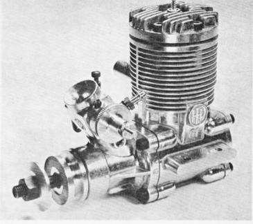
of BDC. Two main transfer ports located fore and aft, angled to direct gas flow to left side of cylinder and timed to open and close at 60 deg. each side of BDC. Third port diametrically opposite exhaust port, angled to sweep gas upward and timed to open and close at 55 deg. each side of BDC.
