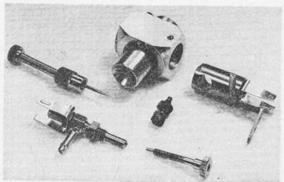
Super-Tigre Mag variant of single-jet 2-needle theme uses sliding rod in spraybar for idle mixture control. Below: Webra TN carburettor. Idle needle (foreground) screwed into barrel, enters jet at low speed to reduce fuel flow.
