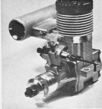
model. The transfer channels are much wider and the cylinder ports are both very much larger and remain open for longer periods. Finally, the carburettor choke area has been increased approximately 30 per cent.
