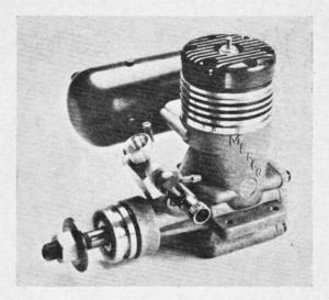
Cylinder-Head. Machined from aluminium alloy bar finned, with black anodized finish. Hemispherical combustion chamber (interrupted by slot for piston baffle clearance) and central ignition plug. Six "Pozidriv" head screws, three extra long and passing through cylinder jacket to secure complete cylinder assembly to crankcase. Paper gasket between cylinder jacket and crankcase. No head gasket.
