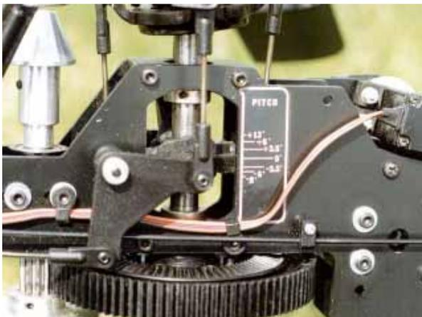
*The 'X-Cell 60' has this pitch gauge included in the decals. If fitted correctly it is quite accurate.*
