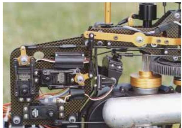
Similarly, there is a push/pull linkage from the tail servo to a bellcrank and then a single pushrod all the way to the tail. Finally, the collective servo has a push/pull linkage to a bellcrank and a single pushrod (actually, it's doubled up with two parallel rods) to the seesaw which moves the swashplate up and down by moving the second bellcrank in the elevator linkage. Before you ask about the lateral cyclic, this has a push/pull linkage from a rocking servo.
