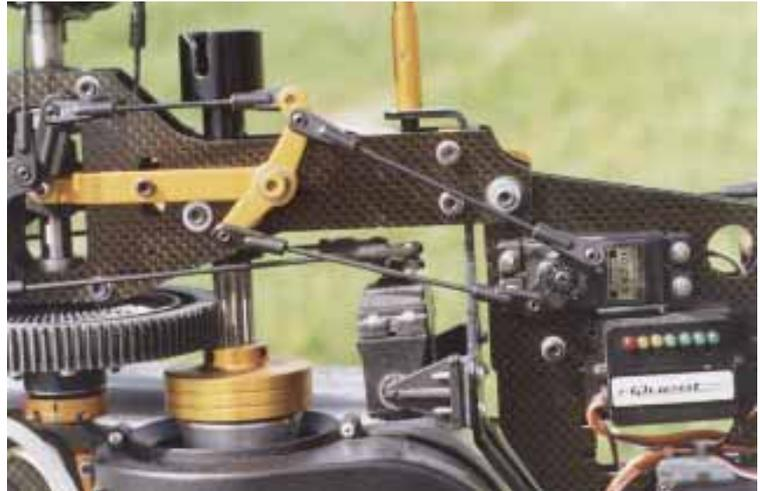
*RH side of the 'Pro'. Note that the elevator push/pull linkage has no offset at the servo arm - as per the instructions. Those protruding screws on the rocking servo mounts do offend me but that's the way they tell you to do it. Note the 'Uni-ball' starter cup, which I like.*
