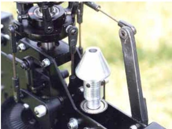
*The cone start on the 'X-Cell 60' is perilously close to both the swashplate front link and the anti-rotation link. It has now been changed to a 'Uni-ball' type as on the 'Pro'.*
