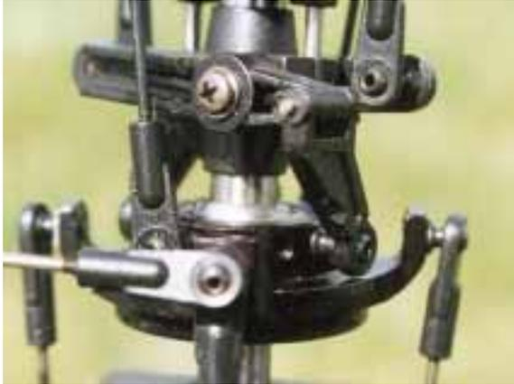
*Look closely and you can see the notch in the mixer link which is needed to clear the swashplate when full cyclic is applied.*
