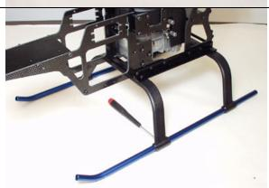
Locate and epoxy the skid pipe tube end caps into the skid pipes.
