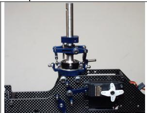
Attach the Anti-rotation Guides Part A & B together using (2) M3-10 Cap Head Bolts.
