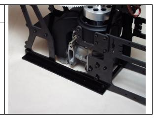
Install (8) M3-12 Cap Head Bolts with (8) M3 Locknuts these nuts and bolts will be installed in the next 4 holes on the frame rails.
