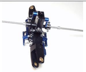
With the rotor head sitting on the head button on the table slide the flybar control arms on each side of the sea-saw with arms in left hand orientation. Measure to insure the flybar is centered as closely as possible and secure the arms to the flybar using (2) M3-3 Set Screws. Also make sure that the arms are parallel to one another.
