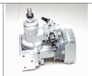
Mount the fan hub to the engine using the Engine collet and the M8 Nord Lock washers. Remove the engines drive washer and replace it with the Brass Collet. Finish attaching the fan hub with (2) M8 Nord Lock Washers under the prop-nut. **Note:** The fan hub must be checked for run out no more than .002"
