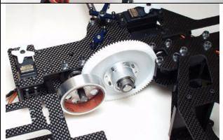
Set Gear mesh between the Clutch Bell and the main-gear as previously described is step 2 of this section.
