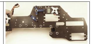
Install the Right Upper Aileron Servo to the Right Upper Frame Using (4) M2.6-14 Cap Head Bolts, (4) M2.6 Lock Nuts & (2) Servo Fixing Plates.
