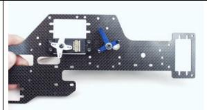
Install the Rudder Servo to the Inside Right Upper Frame Using (4) M2.6-14 Cap Head Bolts, (4) M2.6 Lock Nuts & (2) Servo Fixing Plates.
