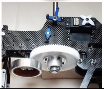
Install the start shaft thru the clutch bell and the bearing block locking it in place using the start coupler and (1) M4-4 Set screw. **Note:** There should be no up or down play once the shaft is fastened in place.
