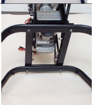
Slide the Skid pipes thru the Struts till you center them to allow adequate support for the helicopter. Fasten the Struts to the skid pipes using (4) M3-3 Set Screws.
