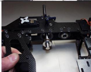
Put the Auto-rotation clutch spacer on the bottom of the main-shaft below the thrust bearing.
