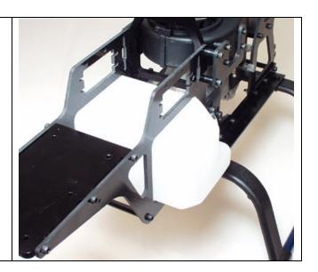
Install mounting plate below tank using (4) M3-10 Cap Head Bolts and (4) M3 Lock Nuts **Note:** For additional support you may want to put a piece of double sided tape onto the mounting plate.
