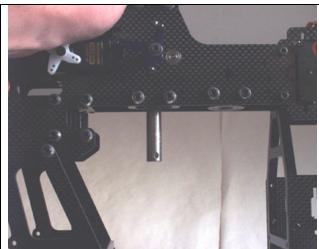
Put the Main Shaft thrust bearing on the lower portion of the mainshaft with the larger hole of the thrust bearing towards the top of the machine.
