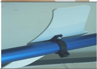
Build the Boom supports using (4) Boom Support ends, (2) Boom Support Rods, & (4) M2-12 Cap Head Bolts. The ends should be parallel to each other and drill a 2mm hole for the retaining bolts to go through and apply a little CA to each end while bolting them together.
