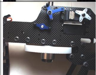
Slide the Main-Shaft collar over the upper portion of the main-shaft Note: there is a ridge on the collar that goes down towards the bearing. Pulls up on the main shaft making sure there is no up or down play then tighten the collar to the shaft using (4) M3-3 set screws.
