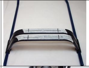
Mount the Struts to the frame rails using (4) M3-18 Cap Head Bolts.
