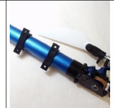
Install the (2) Boom Halves into the frames using (4) M3-35 Cap head Bolts & (4) M3 Lock nut only loosely attach the nuts and bolts.
