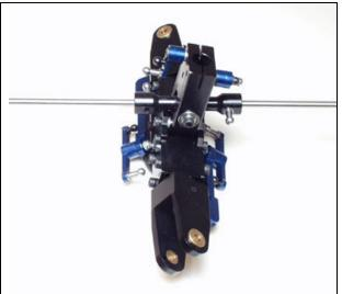
Locate (2) Fly-bar Control arm spacers and slide one on each side of the fly-bar with the ridge of the spacer towards the bearing in the sea-saw.
