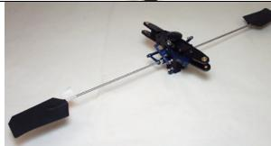
Attach the Completed rotor Head to the Main-shaft using (1) M3-18 Cap Head Bolt & (1) M3 Locknut
