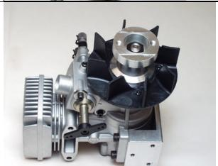
Install Clutch to the fan hub using (2) M4-10 Cap Head Bolts. **Note:** The Clutch must be checked for run out no more than .002" Dial indicate the clutch between the one-way bearing and the clutch shoe.
