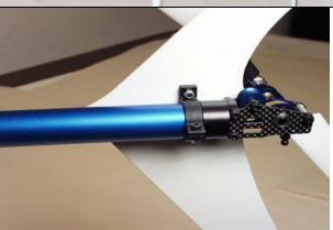
Install (1) Horizontal Fin to other Fin Mount Using (2) M3-10 Cap Head Bolts & (2) M3 Locknuts
