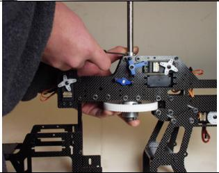
Set the gear mesh between the rear tail transmissions using a double thick piece of notebook paper. Place the paper between the counter gear and the main gear. Loosen the eight bolts that fasten the transmission to the frames and rotate the paper between the gears press the gears together firmly and retighten the bolts and remove paper check for smooth operation of the gears readjust if necessary.
