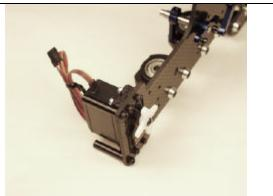
Install the Left Lower Aileron Servo to the Left Upper Frame Using (4) M2.6-14 Cap Head Bolts, (4) M2.6 Lock Nuts & (2) Servo Fixing Plates.
