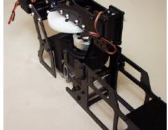
Attach the Shroud to the mounts to the fan Shroud using (8) M2.6-6 Cap Head Bolts.
