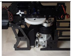
On the right side (Looking from the front of the helicopter) Install Shroud mount using 9mm Cross-spacer and (2) M3-20 Cap Head Bolts.
