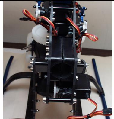
With the belt straight and the Tail rotor Assembly pointed up insert the boom into the boom halves and put the belt over the Front Pulley Gear and pull boom tight to apply tension to the belt
