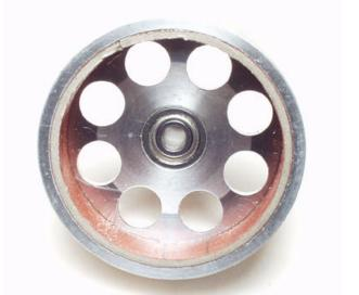
Install the clutch bell into the start shaft-bearing block.
