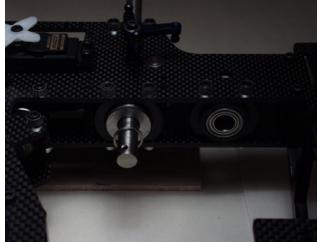
Next put the Auto-rotation clutch on the main-shaft and attach it to the shaft using (1) M3-20 Cap Head Bolt and (1) M3 Locknut.
