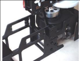
On the Left side (Looking from the front of the helicopter) Install Shroud mount using (2) M3-10 Cap Head Bolts.
