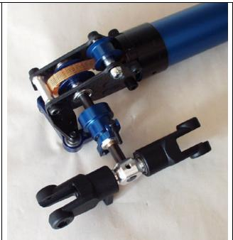
Install (2) 5mm Tail Rotor Blades Using (4) Tail Rotor Blade spacers, (2) M3-18 Cap Head Bolts, (2) M3 Lock Nuts.
