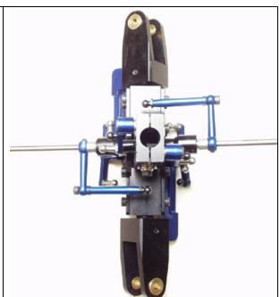
Install M4 Paddles on each end of the fly-bar threading them on 15mm on each side.
