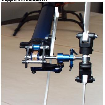
Adjust the Fin parallel to frame set and lock it down using (1) M3-12 Cap Head Bolt & (1) M3 Locknut
