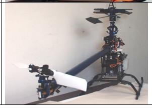
Rotate the Tail rotor down to a 90 degree position and make sure the belt is tight and tighten the four bolts that hold the boom Halves
