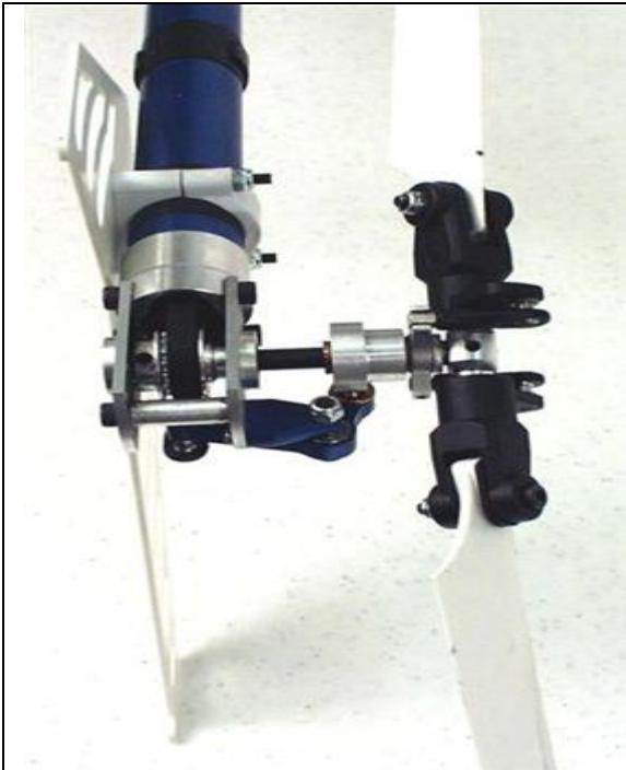
Picture 7, Tail Negative Thrust
