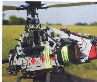
The four-cell Futaba NR-4RB 1,000mAh NiCd radio battery is mounted on the forward right side of the heli's frame.
