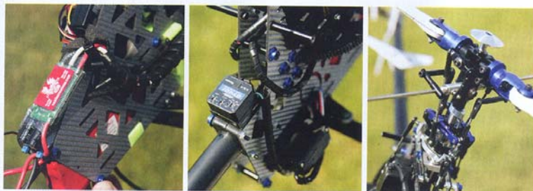
Left: Castle Creations Phoenix 80 speed control fits nicely on the carbon fiber frame. Middle: Futaba GY401 S.M.M. rate gyro. Right: the main rotor head featured high-quality machined parts.
