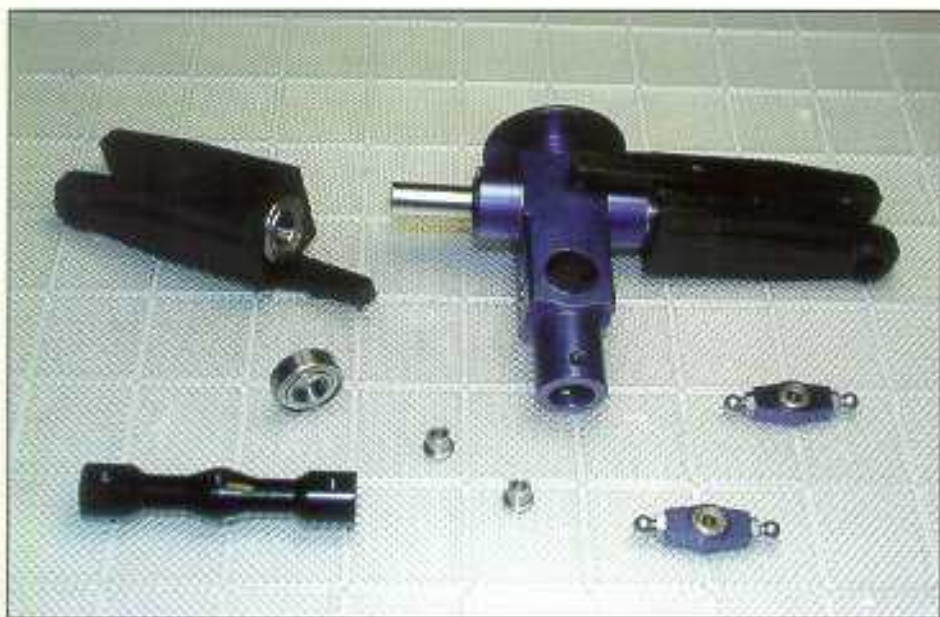
Break down view and construction of the main rotor head. The Learner uses a single axle type design. A "palm brake" is machined into the hub block.
