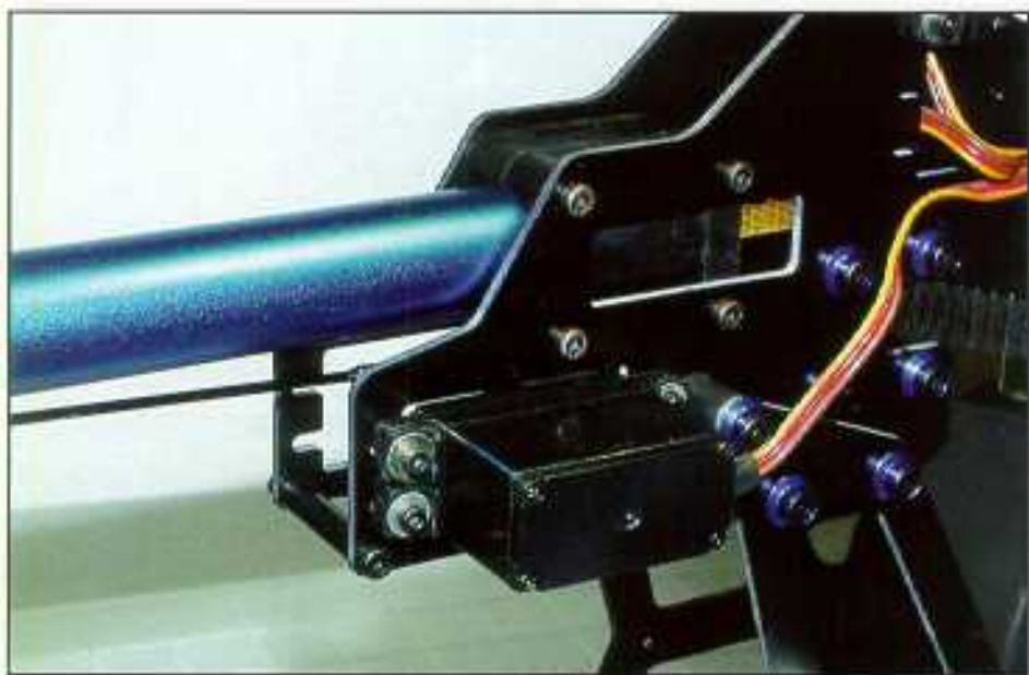
Note simple modification to the tail rotor. The servo is turned 180 degrees from the recommended position. This allowed the servo lead to reach the receiver without an extension. Also note the clean appearance. Carbon push rod was long enough to accommodate the change.
