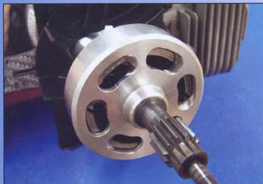
Image shows the GasHer's clutch and pinion arrangement.
