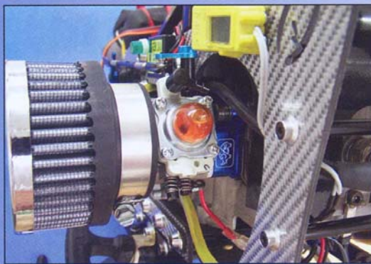
Note carburetor and Z-RC's machined aluminum spacer - see text.
