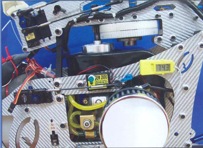
Side view shows the modular construction. Note the dual gear drive train. Plenty of room for the radio gear.
