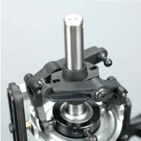
6B.2 - Install Washout Mixer
