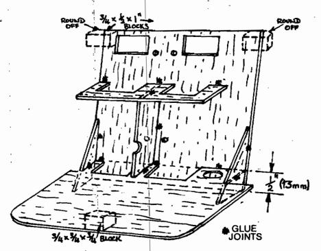
ASSEMBLY OF MAIN PLYWOOD CABIN
