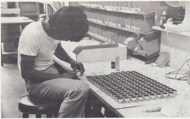
ALL OUR CLUTCH BELLS ARE TESTED AFTER ASSEMBLY BEFORE GOING INTO KITS
