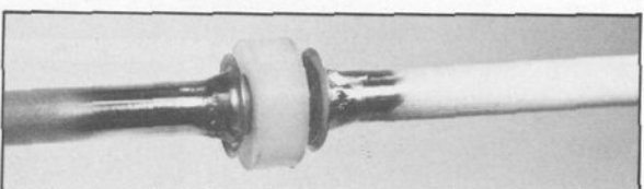
ABOVE, LEFT: Tail rotor gear box drive connector soldered to brass drive shaft. ABOVE: Close-up of one of two teflon bearings soldered to drive shaft. Use 1/16" thick balsa spacers on each side of teflon bearing as soldering aid. LEFT: Front bearing block and gear fitted to drive shaft. BELOW: Completed drive shaft and tail boom ready for installation.
