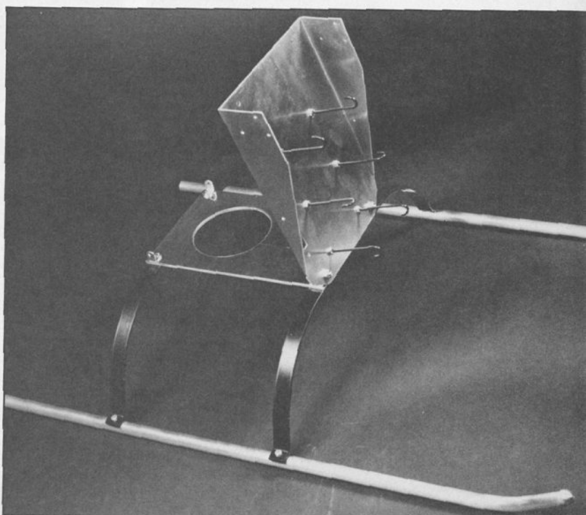
Belt tension spacer under motor lugs and throttle tube guide shown at left. Cut-outs made in gear cover above.
