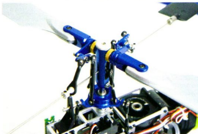
Keeping it simple - moving the flybar system works well and keeps the part count down
