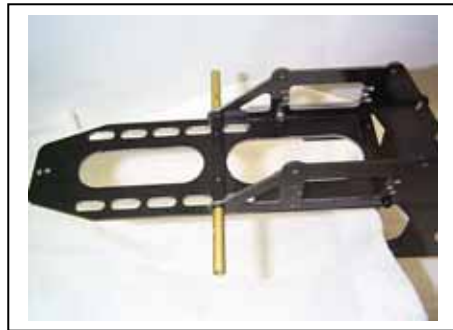
Battery Tray Installed, Top View
