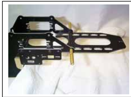
Switch & Gyro Switch Tray Installed
