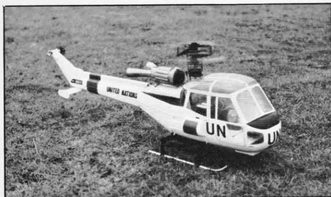
Not the best photo we've taken but it does clearly show where we put the tail servo. This position makes for a good straight-ish and short run and the servo lead is long enough to reach the gyro box. The method recommended by Morley Helicopters — but not shown on the plan — takes the pushrod along a very tortuous route and would have made dismantling the model very difficult. Our way you just unplug the servo.
