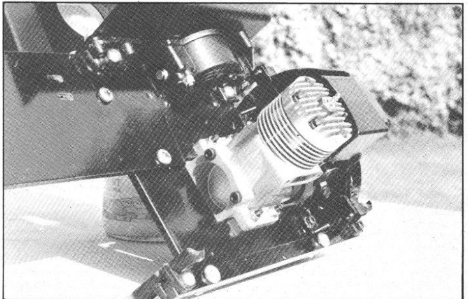
Engine side of basic frame, note the bracketry holding it all together, and the cooling duct arrangements.
