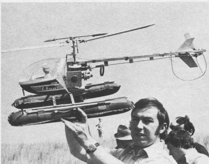
Above: Joe Stafford's modified Lark uses O.S.40 power and square section tail boom. Note the number of supports along the boom for the rear rotor drive. Large heat sink to dissipate heat seen in close-up top right.
